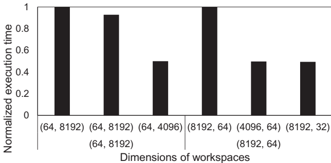
Fig. A.1 . Normalized kernel execution times of workspaces.
